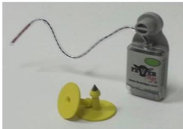
The tag will flash brightly if the calf’s temperature continuously exceeds 39.7°C for 6 hours (settings are adjustable).
